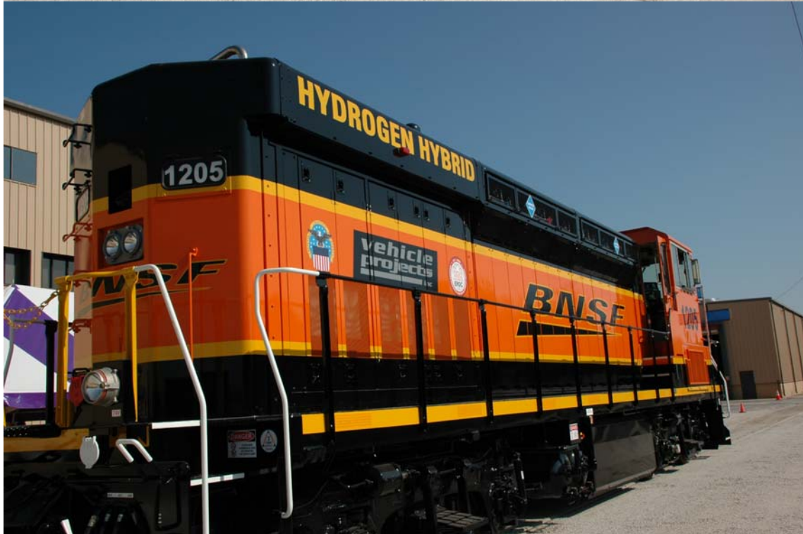
Fuelcell switch locomotive: This is the largest fuelcell land vehicle, photographed at a press conference in completed form on 29 June 2009. Fueled by hydrogen, the locomotive's job is assembling and disassembling trains in urban railyards, where its quiet and zero-emission operation is beneficial. In collaboration with BNSF Railway Company and the US Army, the vehicle was developed by Vehicle Projects Inc of Golden, Colorado, USA. Copyright © 2010 by Vehicle Projects Inc
