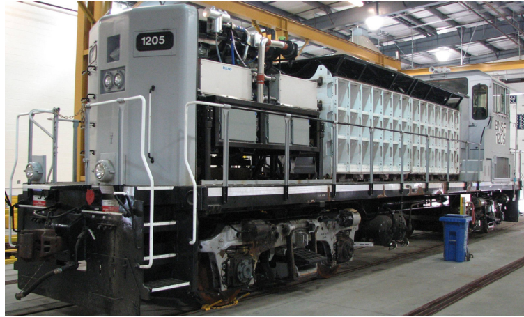
Fig. 2. Locomotive under construction: Right-rear view of the locomotive with installed fuel-cell prime mover shown in the foreground (31 July 2008)
