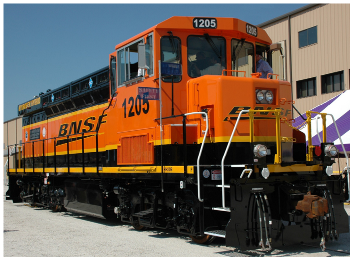
Fig. 1. Fuel-cell switch locomotive: This is the largest fuel-cell land vehicle, photographed at a press conference in completed form on 29 June 2009.
