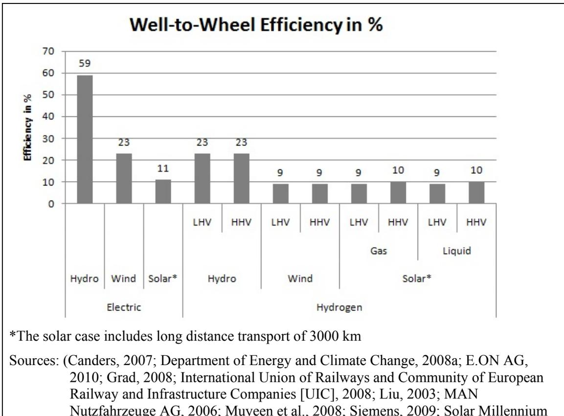
In the case of hydro and wind the losses of the electric system are significantly lower than in the hydrogen system. The available areas to build new hydro power plants are limited. Hydro electricity may, therefore, not be available for electrification plans of railways. The solar efficiencies over a distance of 3000 km are similar between the electric- and the hydrogen systems.
