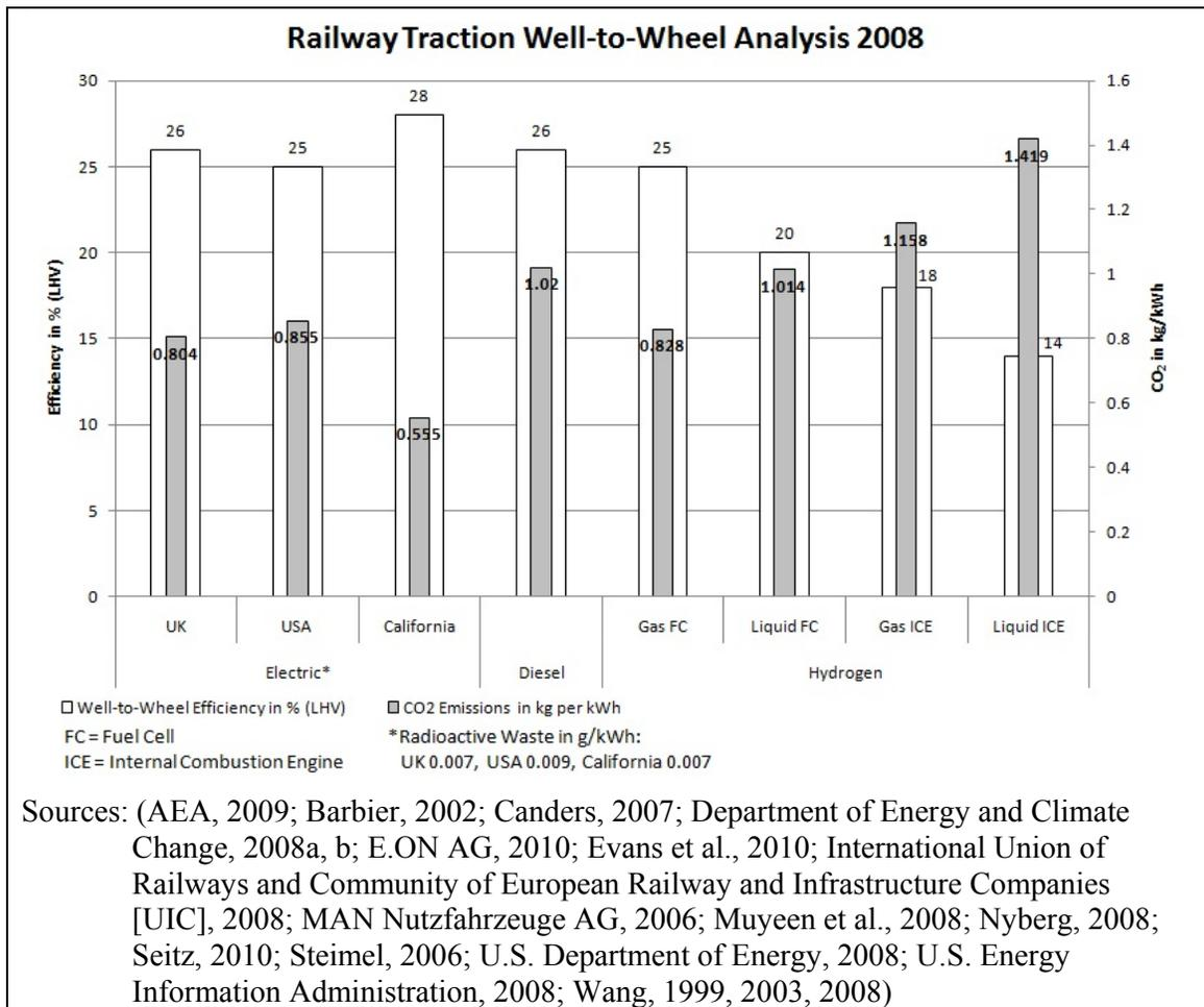
Figure 3: Railway Traction Well-to-Wheel Analysis 2008 based on the HHV
